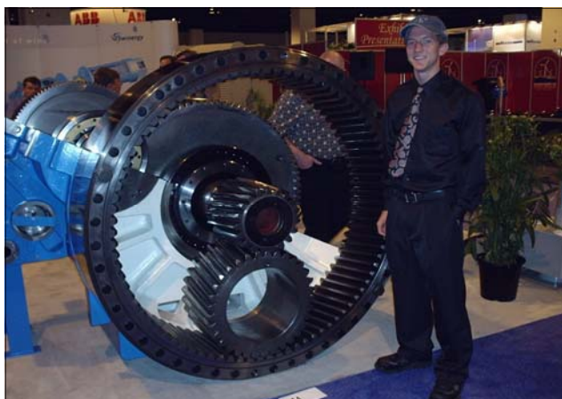
Left: Sean Kissinger stands next to the gear that turns wind turbine blades to feather against the wind.
